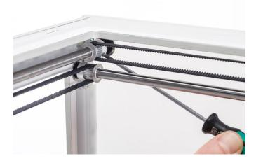
The axles should not move at all. If one of the axles does move, you can observe a ticking noise of the pulleys hitting the frame. In this case it is recommended to calibrate the print head. For instructions on how to do this, take a look at the <u>Ultimaker website</u>.
