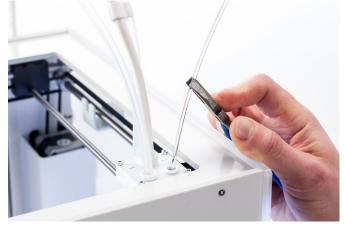
6. Take a look at the tip of the filament and see if it has a clean, cone-shaped tip like shown on the example to the right.
