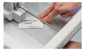
After calibrating the build plate with the first nozzle, the second nozzle needs to be aligned as well, to ensure the heights of both nozzles are set correctly. For this it is only necessary to set the correct height by using the calibration card.
