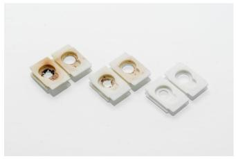
According to these images, it is highly recommended to replace the cover on the left and advisable to replace the cover in the middle. The cover on the right is in perfect condition and will not need to be replaced. Instructions on how to replace the silicone nozzle cover can be found on the <u>Ultimaker website</u>.
